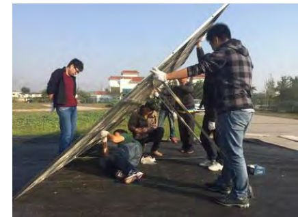
Fan-shaped target was deployed with its face perpendicular to the line of sensor sight
