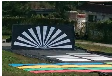
Fan-shaped target was deployed with its face perpendicular to the line of sensor sight
