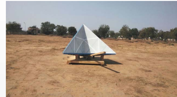
Deployed Perforated CR
