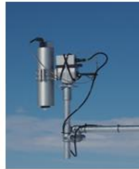
HYPSTAR® system [https://hypstar.eu/] 380-1700nm, 3-10nm FWHM
