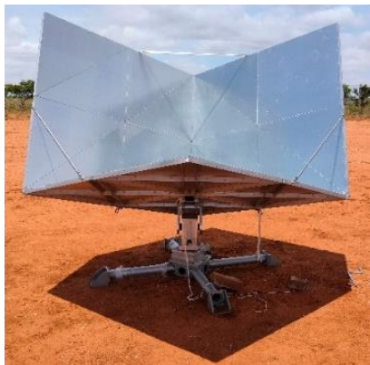
Corner reflector designed & developed for NISAR mission deployed
