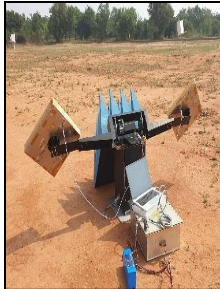
Corner reflector designed & developed for NISAR mission deployed
