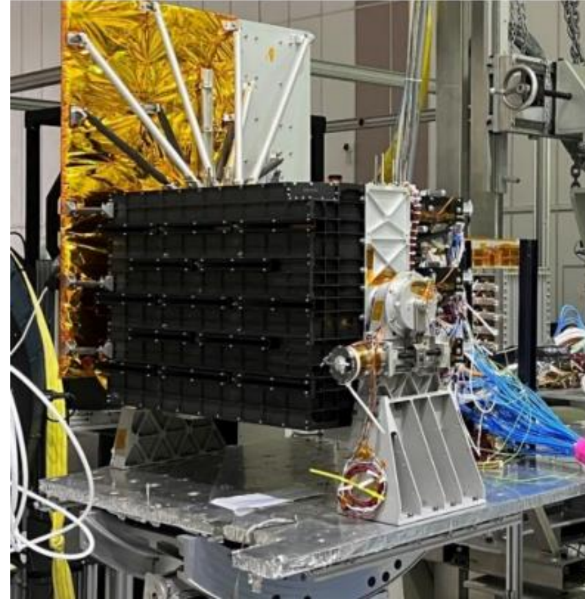
OCM-3 payload Electro-Optical Flight Module
