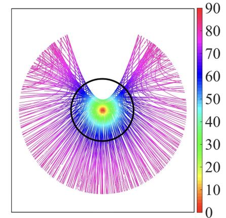
Scheme of ground-based GNSS-MR sea-level estimation. The distribution of 48-hour specular reflection points are drawn and the color varies with the incident angle as the right legend.
