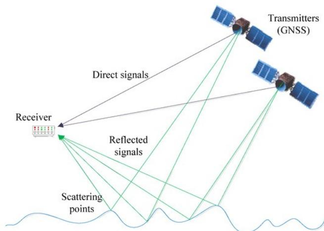
The ocean surface roughness measured by GNSS-R is represented as mean square slope (MSS) modulated by the wave spectrum and signal's wavelength
