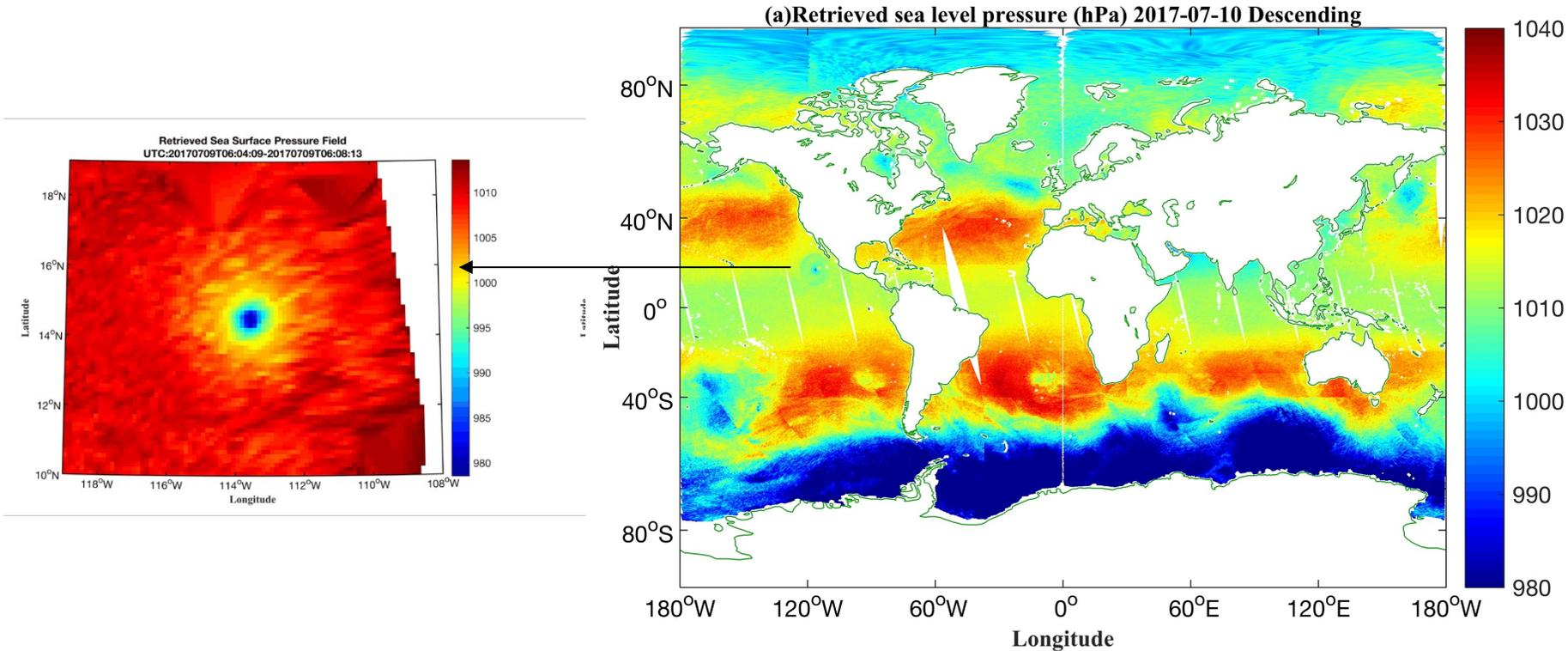
A set of all-weather (clear-sky, cloudy, rainy and high wind conditions) ocean surface pressure retrievals from joint observations of FY-3D/MWTS-II and FY-3D/MWHTS
