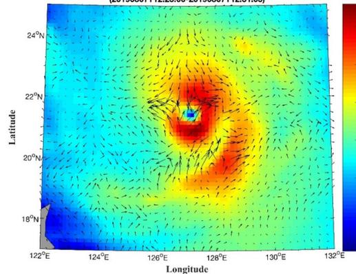
Retrieved surface pressure gradient (vector) and GDAS wind field (shading)
