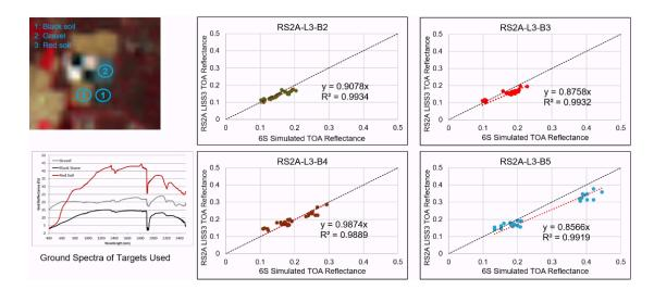
A degradation in TOA reflectance has been observed in the B5 band, which is being addressed in the data products. Cross-calibration between RS2A and Landsat-8/9 OLI showed a good alignment.
