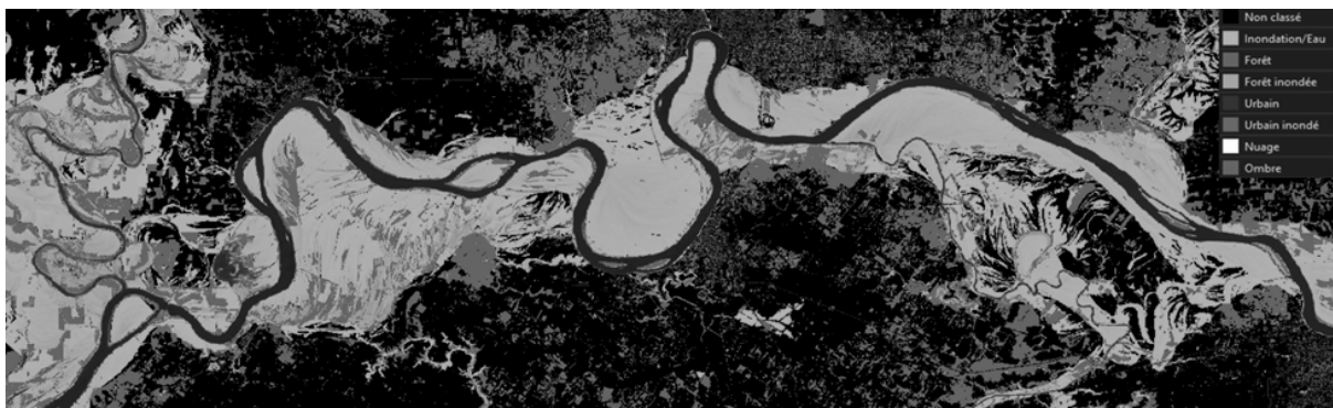
Figure 5.2.3-1 FloodML flood extent map from Sentinel-2 data, ESA World Cover and GSWO over the Ohio River flood event on the 27th February 2018
