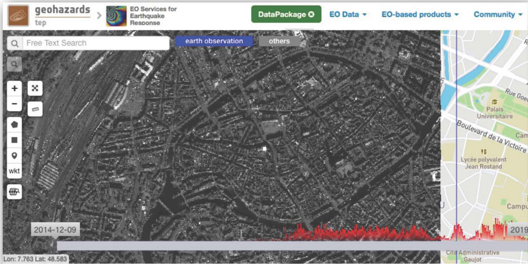
Ortho-images of a HR-DSM (0.5m) over the city of Strasbourg / Pléiades stereo of Sept. 2016
