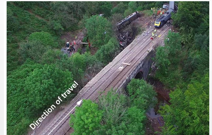
Landslide-induced train derailment at Carmont (UK/Scotland) – August 2020
