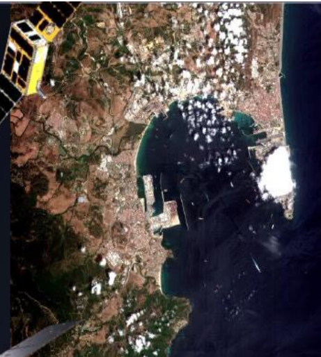
PhiSat-2 data showing the Bay of Gibraltar. True colour image at a resolution of 4.8m per pixel
