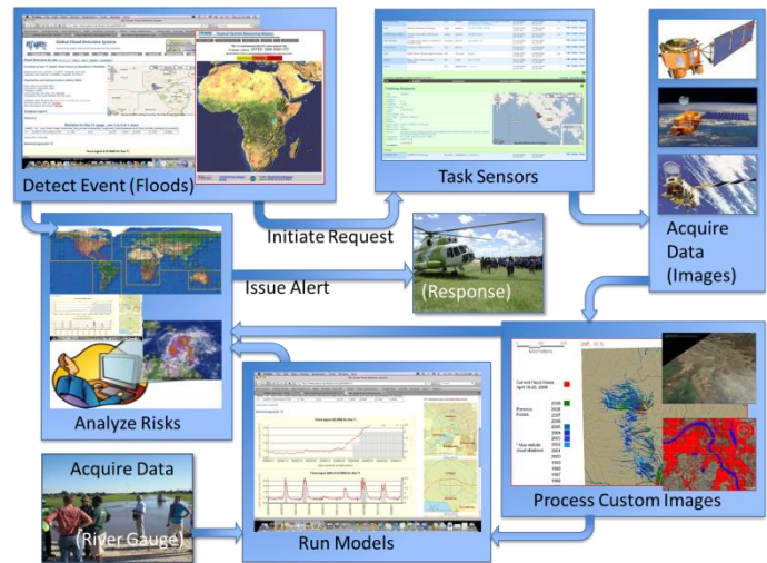
Figure 9. Namibia Flood Pilot: data flows and information processing
