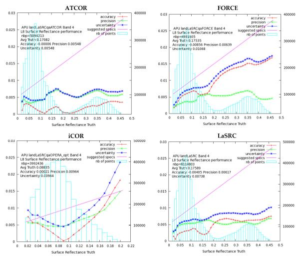
The accuracy (red line), precision (green line), and uncertainty (blue line) as computed in bins (blue bars) for OLI Band 4 (Red). The total number of pixels (nbp) used in the computations is given also in the plot. The magenta line represents the theoretical SR reference for Landsat SR ( $0.005+0.05\times\rho$ ).
